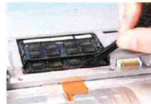
You'll hear a click when you slide in the RAM, but use your black stick to be sure it's in.
