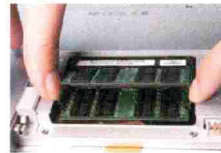
Use your thumbs to spread the tiny metal tabs to remove the RAM.
